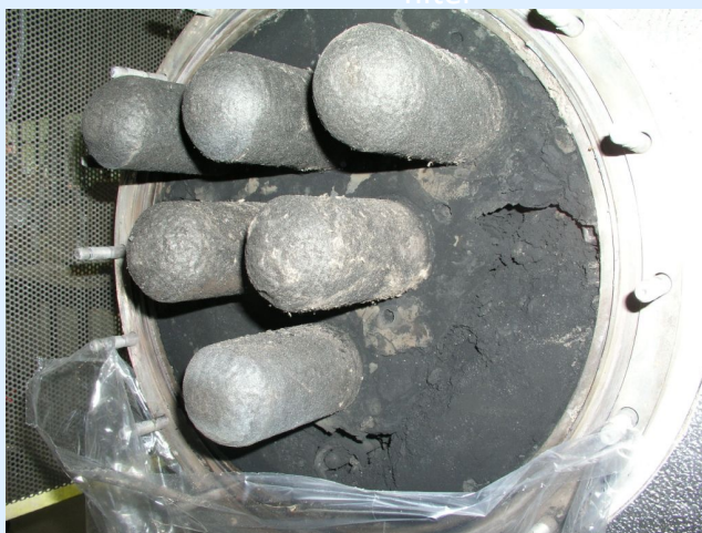
Raw gas chamber completely filled with ash (2 kg)
