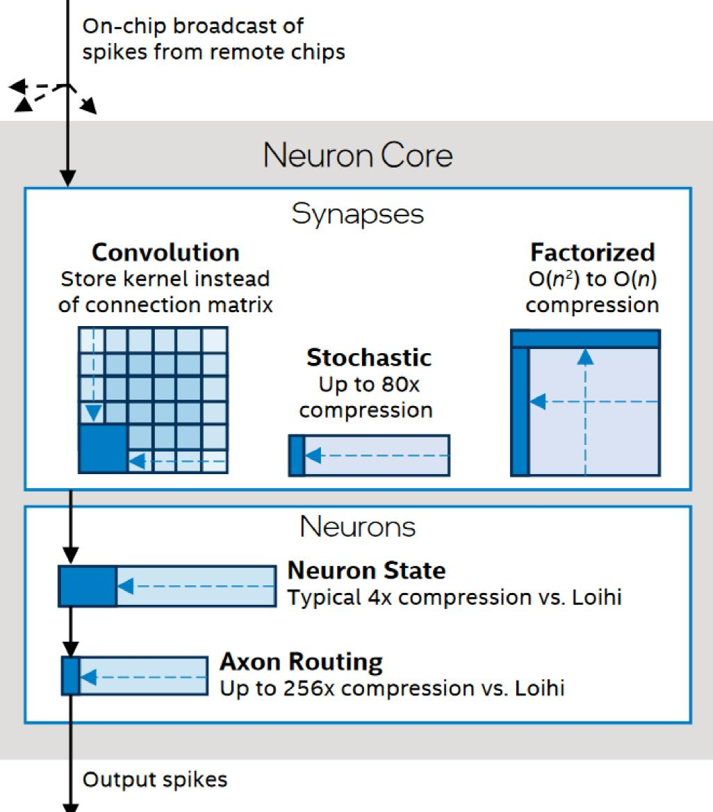
Apart from spike broadcast (as opposed to targeted delivery lines), the chip also implements features such as weight matrices compatible with convolutional neural networks and outer-product weight matrices (factorial, see conv-net lecture).
