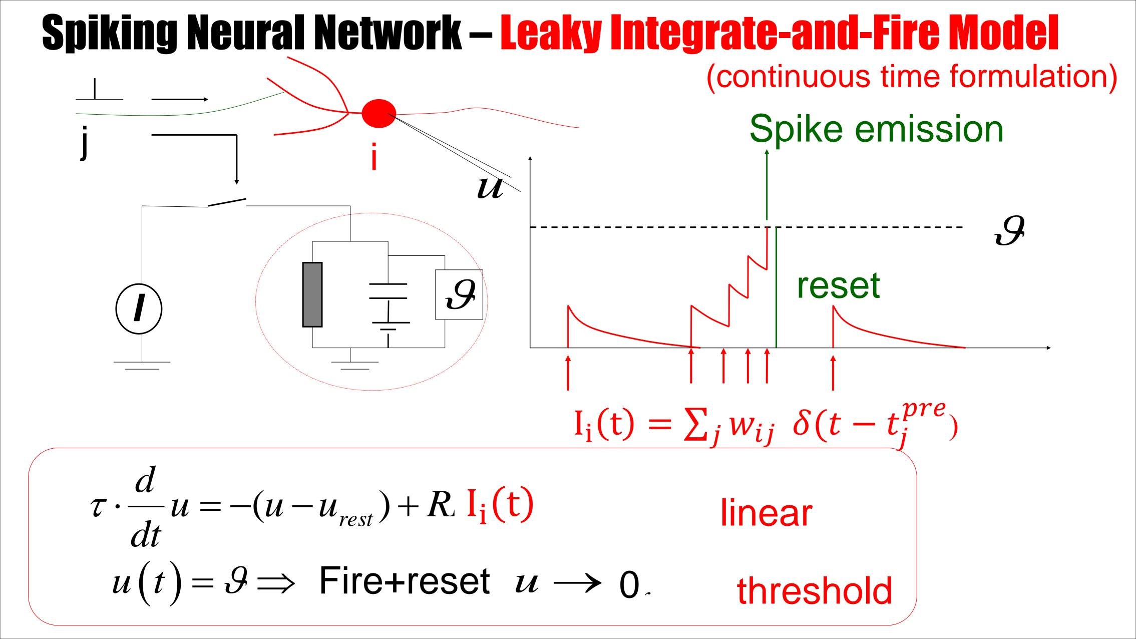
The Leaky integrate-and-fire model written in **continuous time** involves a LINEAR differential equation that can be interpreted as an electrical RC circuit charged by a current I(t). This current I(t) consists of short electrical pulses that present spike arrivals. The  $\delta(t - t_i^{pre})$ denotes the Dirac delta function for each presynaptic spike arrival at times  $t_i^{pre}$  and  $w_{ij}$  are the weights.
