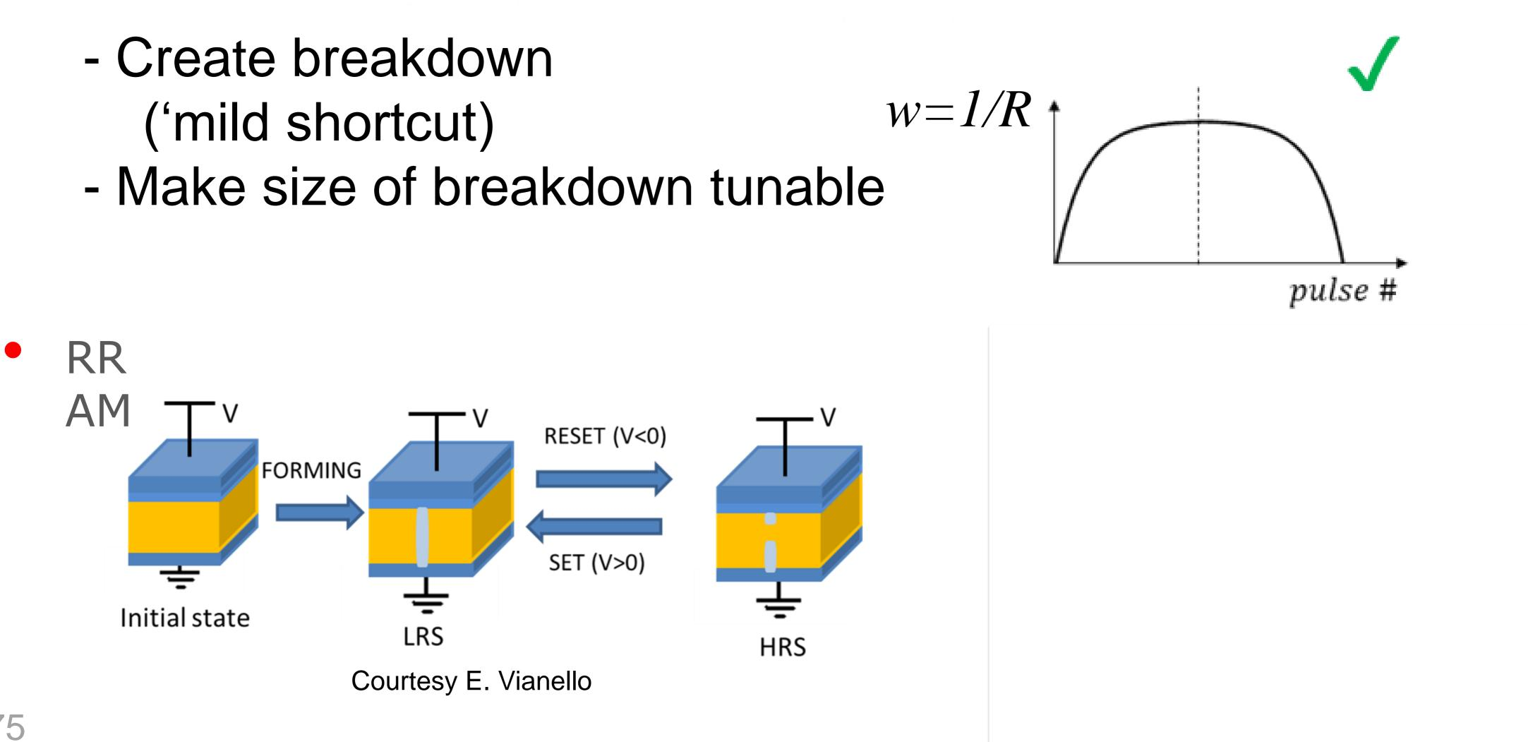
Here The material in yellow is an electrical insulator (dielectric material). However, with a first strong voltage pulse one can create an initial breakdown (blue channel) in the material.
