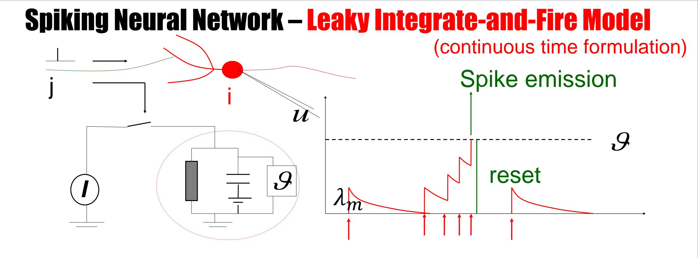
$$\begin{array}{lll} \Delta u_{i} = w_{ij} & if \quad t = t_{j}^{pre} \\ u_{i} \leftarrow \lambda_{m} u_{i} \\ if \quad u_{i} = \vartheta \quad u_{i} \leftarrow 0 \end{array} \begin{array}{ll} \text{Linea} \\ \text{Thres} \end{array}$$
