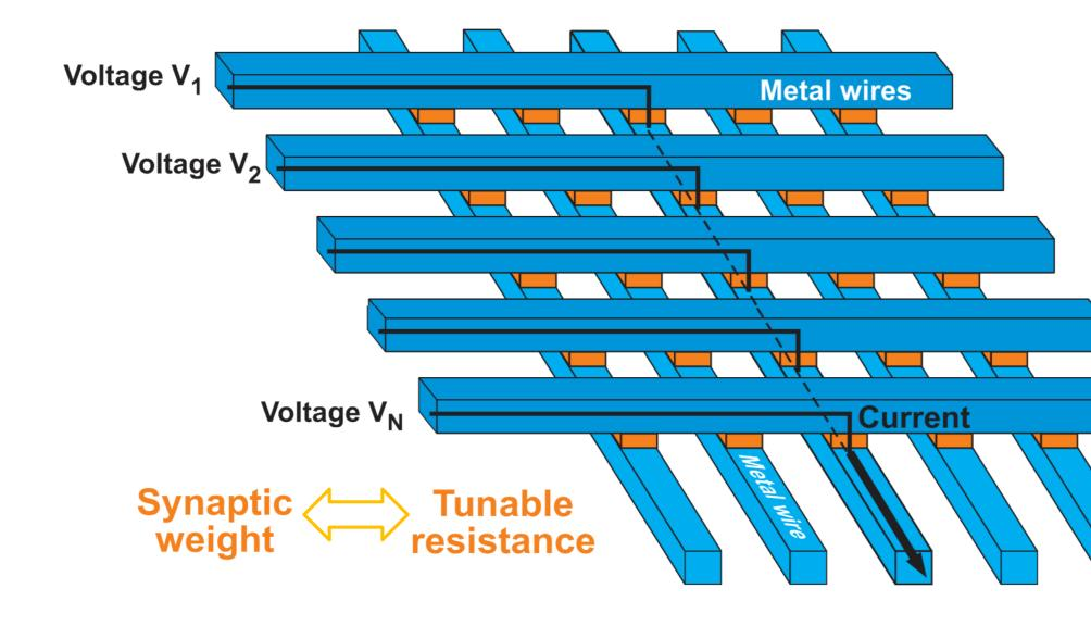
Input signal  $x_i = V_i$  voltage of neuron j Weight  $w_{ij} = 1/R_{ij}$  resistor at crossing Output  $I_i = \sum_j \frac{V_j}{R_{ij}} = \sum_j w_{ij} x_j$  current into neuron i
