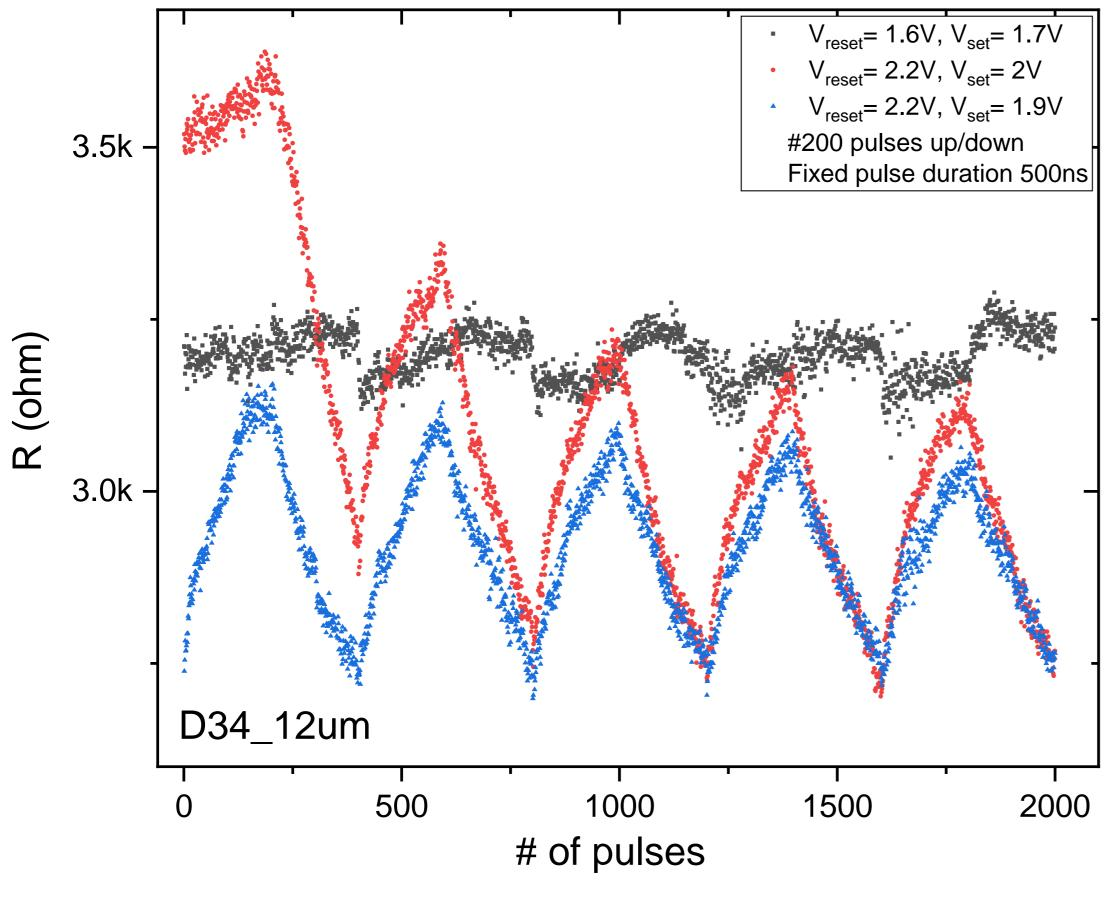
Experimental demonstration of symmetric and continuous change of G
