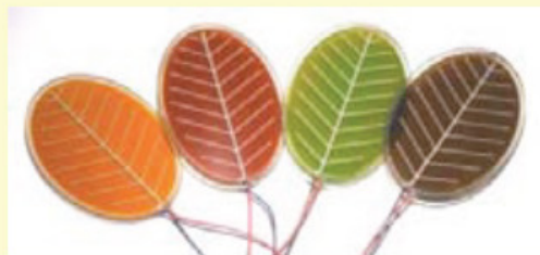
Leaf-shaped transparent DSC with four colors
