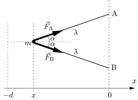
$$m\ddot{x} = F_{A,x} + F_{B,x} = -4kx = -\frac{F_{\max}}{d}x \quad (10)$$
