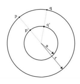
The granitational force on a body that lies outside a spherical shell of matter is the same as it would be it all the shell's matter were concentrated into a point at its center
