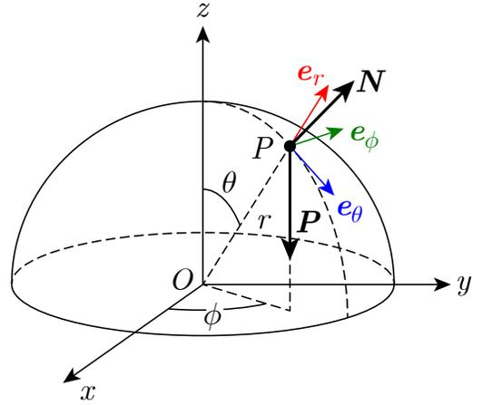
$$\mathbf{a} = -R(\dot{\theta}^2 + \dot{\phi}^2 \sin^2 \theta) \mathbf{e}_r + R(\ddot{\theta} - \dot{\phi}^2 \cos \theta \sin \theta) \mathbf{e}_\theta + R(\ddot{\phi} \sin \theta + 2\dot{\phi}\dot{\theta} \cos \theta) \mathbf{e}_\phi.$$
