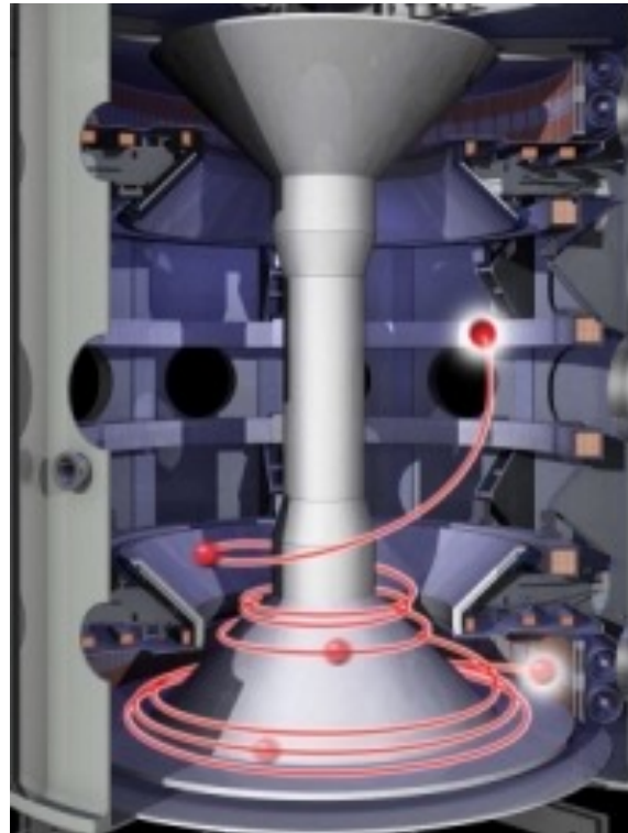
Super-X divertor MAST-U (UK)
