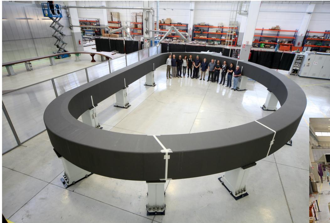
Toroidal Field coils
