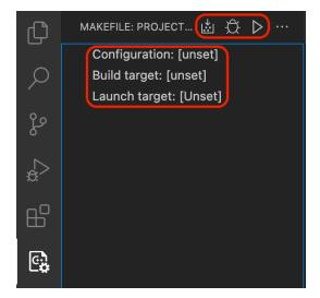
There are three buttons on the top side of the window, respectively corresponding to the *build*, *debug* and *run* commands, which are quite similar to the "Run and Debug" function of *VSC* that is already introduced in Section 3. Additionally, there are three different items of configurations: *Configuration*, *Build target* and *Launch target*, by customizing which we can instruct *VSC* to make use of the Makefile in the way we want.
