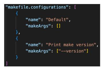
One more *make* command configuration, *Print make version*, now becomes available, which adds the "–version" argument to the make utility. With this make command configuration, every time we build our program using *Makefile Tools*, the version of *make* would be printed out. In my case, the following information is displayed in the terminal:
