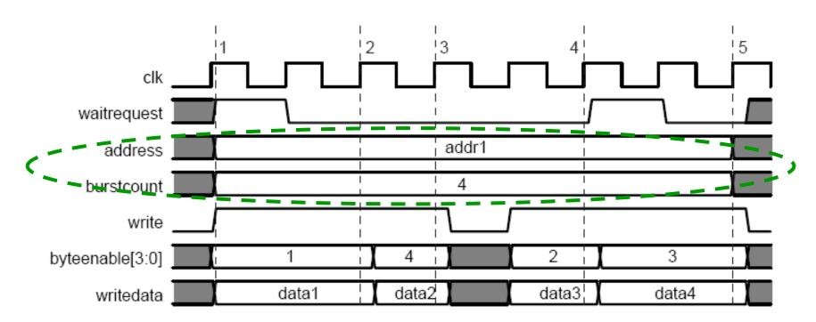
Address and BurstCount available for the whole transfer Write can be deactivated by the master The number of burstcount needs to be generated
