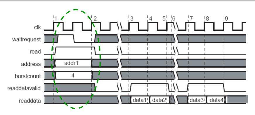
Address and BurstCount available for the first cycle only Read signal only for the first cycle The number of burstcount ReadDataValid needs to be generated The master could start a new transfer in 2
