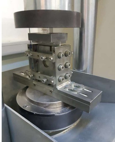
Figure 5: CAI holder based on Boeing BSS 7260.
